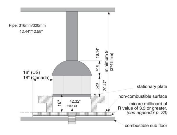
A MINIMUM CLEARANCE OF 16" FROM THE FLOOR TO THE TOP OF THE STATIONARY PLATE STRICTLY MUST APPLY.
