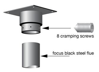
the order to tightening the plate screws (to secure progressively)
