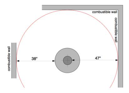
Wall clearances with optional blocking mechanism:
