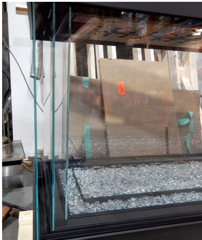
Figure 100. Glass installed (side view - no gaps)
