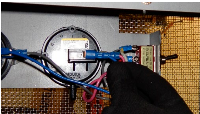
Figure 112. Disconnect blue wire.
