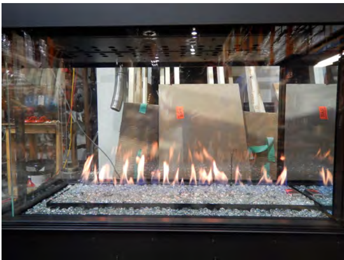
Figure 101. Test flame (side view)
