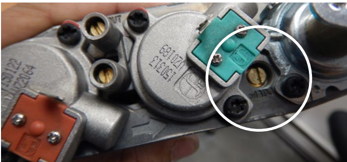
Figure 13.g Adjust pilot size
