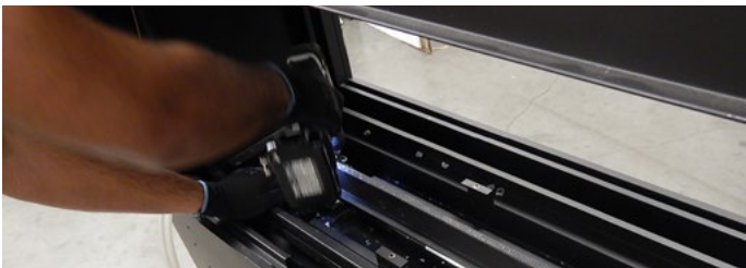
Figure 12.d Removing the Burner screws
