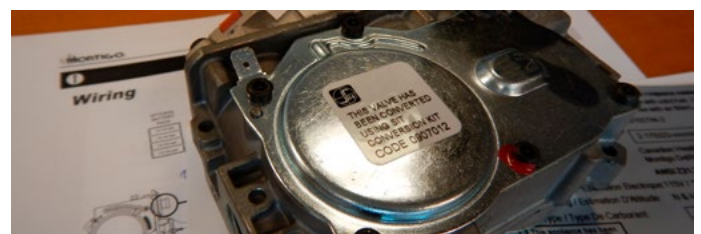
Figure 13.k Conversion label on valve
