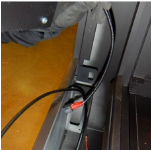
Figure 24.e On/Off switch through drawer
