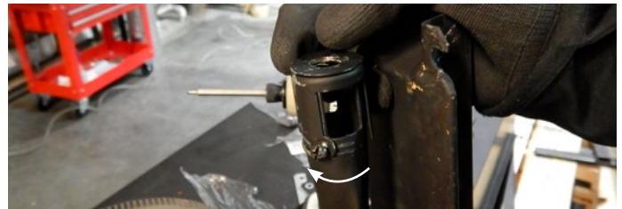
Figure 13.b Loosening the venturi
