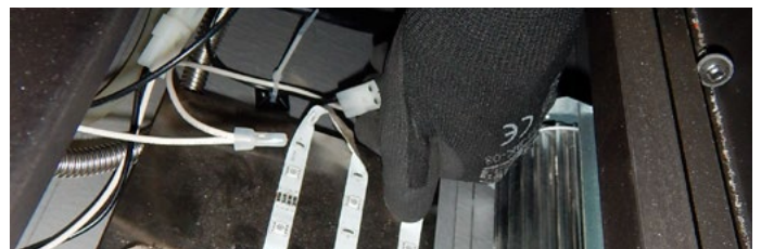
Figure 27.f Connect control board connector
