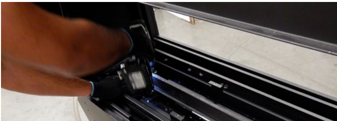
Figure 12.d Removing the Burner screws
