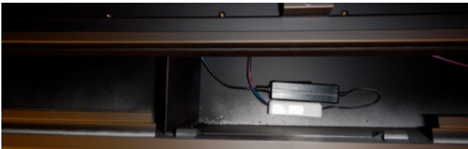
Figure 25.a. Secure LED receiver
