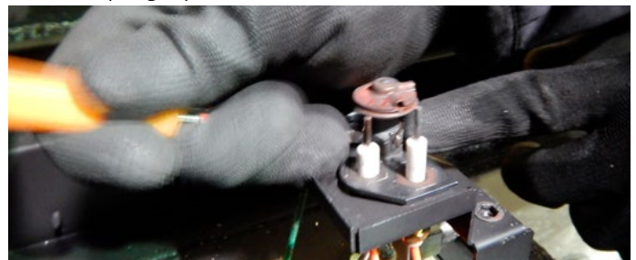
Figure 13.d Removing the spring clip
