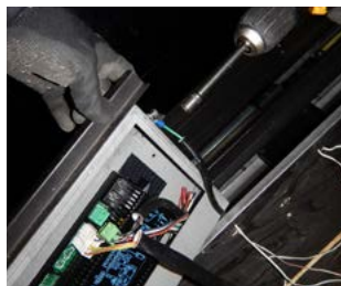
Figure 24.b Remove existing basic board
