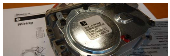
Figure 13.k Conversion label on valve
