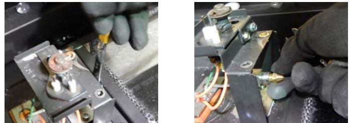
Figure 13.c Removing the orifice
