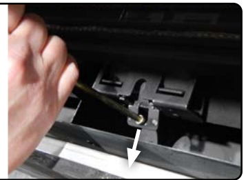
Figure 21.d Pull door latches
