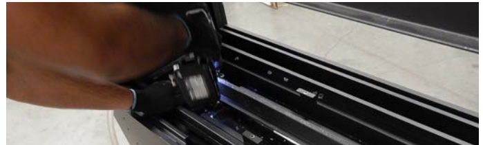
Figure 13. Removal of burner strip
