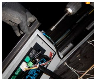
Figure 24.b Remove existing basic board
