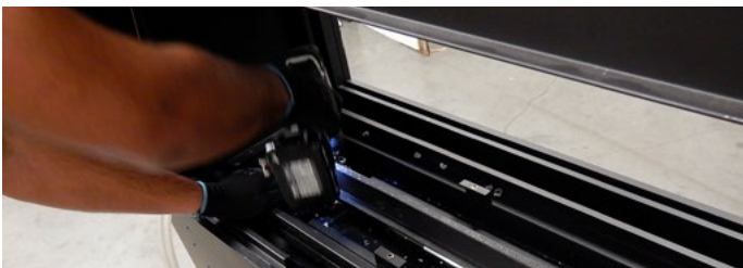
Figure 12.d Removing the Burner screws
