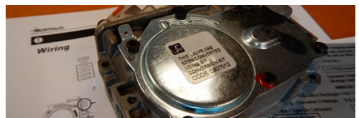
Figure 13.k Conversion label on valve
