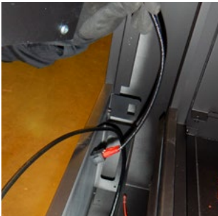
Figure 24.e On/Off switch through drawer
