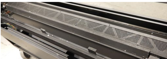
Figure 12.c Removing the media trays
