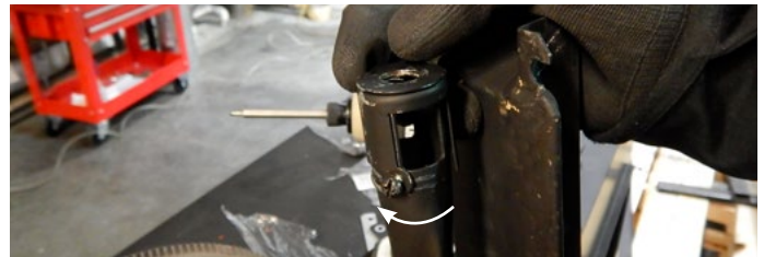
Figure 13.b Loosening the venturi
