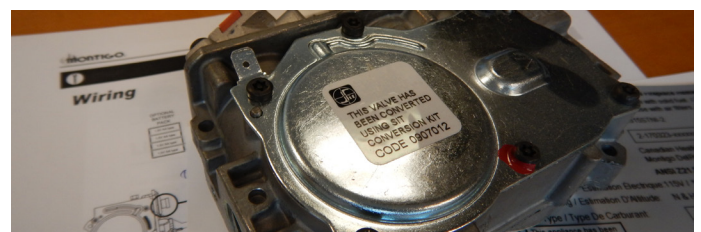
Figure 13.k Conversion label on valve
