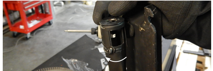
Figure 13.b Loosening the venturi
