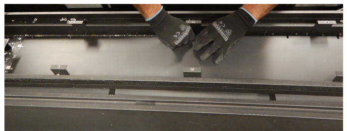
Figure 12.g Removing metal plate
