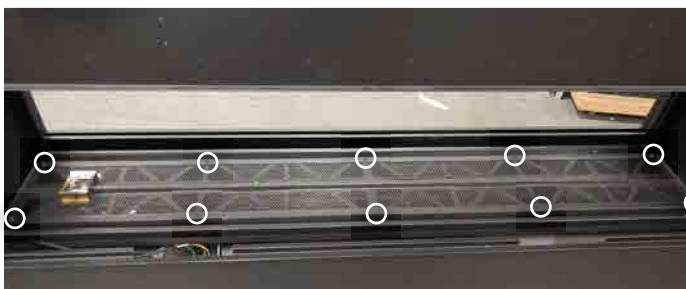
Figure 12.b Unscrewing the media trays
