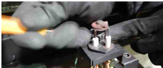
Figure 13.d Removing the spring clip
