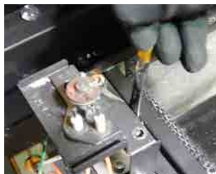
Figure 13.c Removing the orifice
