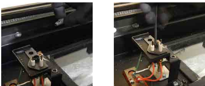
Figure 13.f Insert propane orifice, reassemble burner
