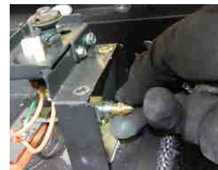
Figure 13.c Removing the orifice
