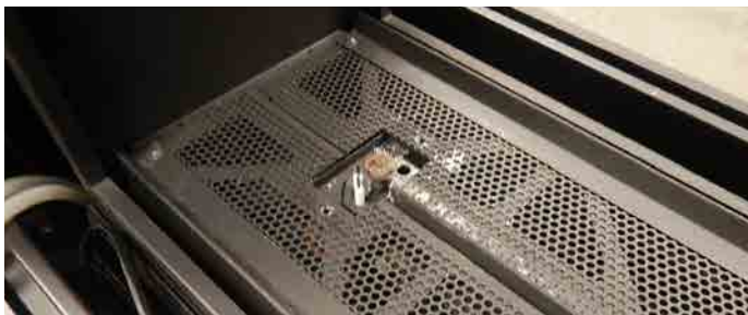
Figure 12.a Removal of the pilot cover
