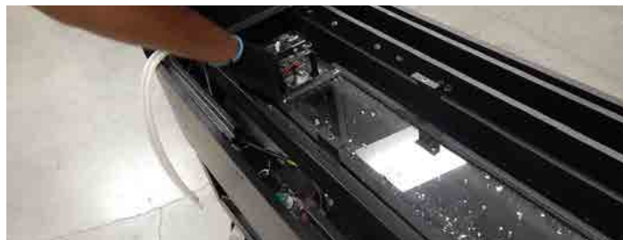
Figure 25.d Insert glass plate
