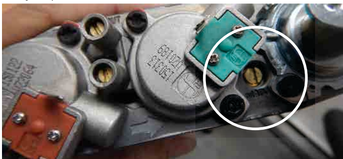
Figure 13.g Adjust pilot size
