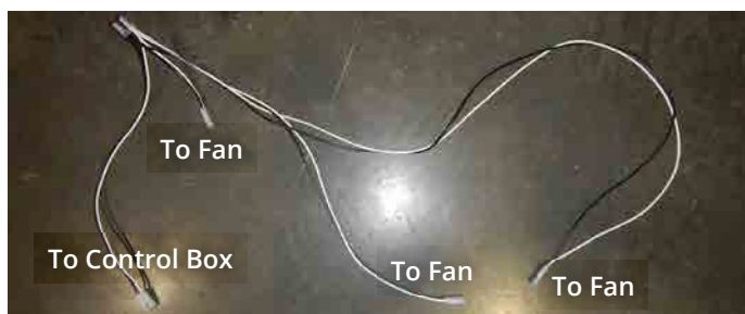
Figure 27.e Locate fan wiring harness
