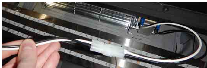
Figure 27.g Connect fans to harness connectors
