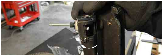
Figure 13.b Loosening the venturi
