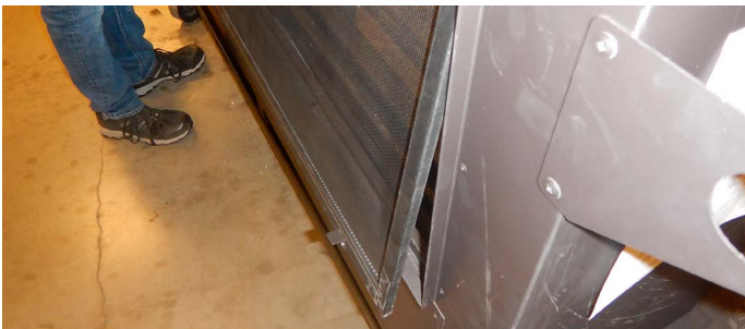
Figure 20.b Lift out the Retaining Tabs and screen
