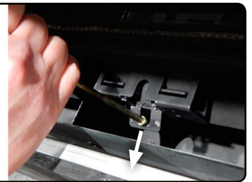
Figure 21.d Pull door latches
