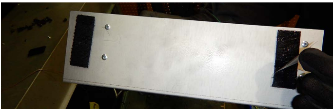
Figure 27.b prepare velcro strips
