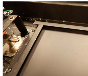
Figure 12.f Unscrewing brackets securing metal plate
