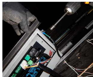
Figure 24.b Remove existing basic board
