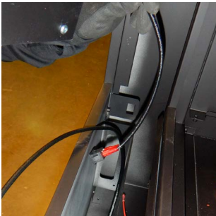
Figure 24.e On/Off switch through drawer
