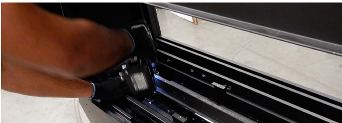
Figure 12.d Removing the Burner screws
