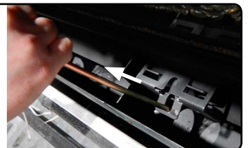
Figure 21.d Pull door latches
