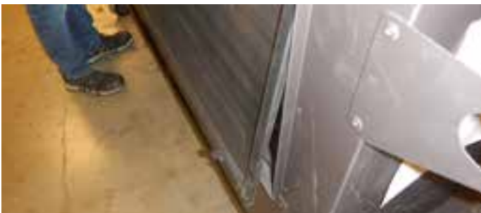
Figure 20.b Lift out the Retaining Tabs and screen
