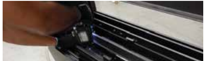
Figure 13. Removal of burner strip
