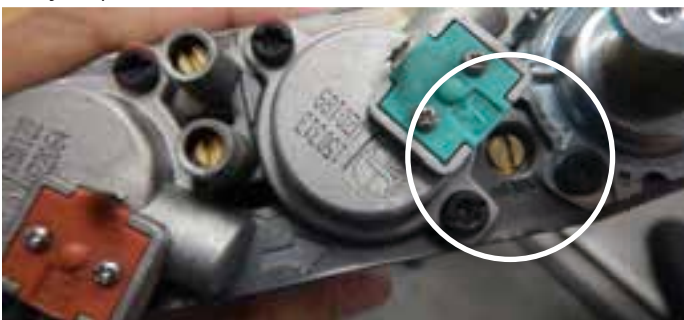
Figure 13.g Adjust pilot size
