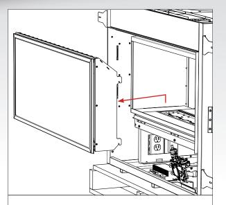
2) To aid in the installation of your surround remove the safety screen by lifting it up off the hooks and pulling the screen assembly out.
