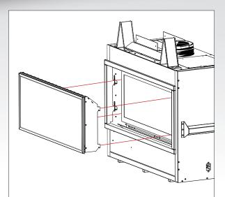
5) Reinstall the safety screen by inserting the four tabs on the back of the screen into the four slots further back in the stove.
