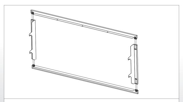
1) Using the M5 screw and nuts provided. Attach all four pieces as shown in the picuture above, use a 4mm allen key to tighten the screws. Make sure the notches on the left and right pieces face downward and the top piece has the slots.
