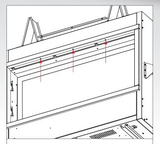
6) If surround starts to warp after usage, use self-tapping metal screws (not included) in the slots located on the underside of the top surround piece. (screen removal required, see steps 2 and 5)
