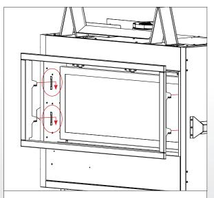
4) For C34, C60, and C72 models insert the notched tabs on the surround into the forward most slots in the stove (circled above).
