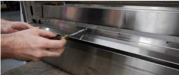
Figure 4 Removal of lower air baffle
