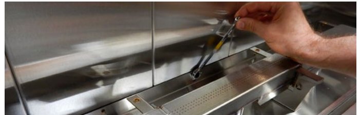
Figure 52 Loosening air baffle bolts
