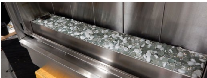
Figure 67 Spreading the firestones evenly and make sure there are no firestones covering the pilot.
