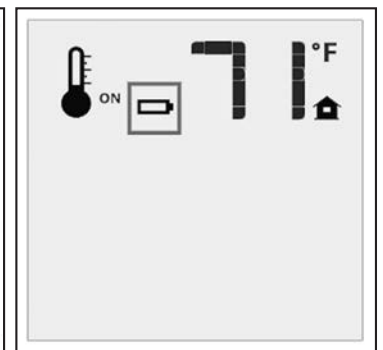
Figure 16: Low Battery Indicator.
