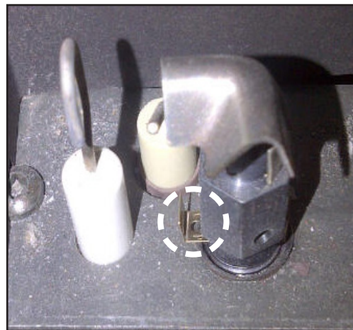
Figure 23. Pilot Slider set to LP
