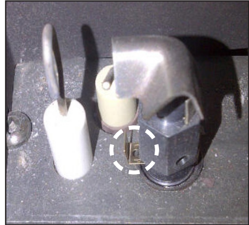
Figure 20. Pilot Slider set to LP
