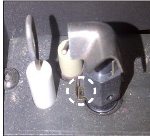
Figure 20. Pilot Slider set to LP
