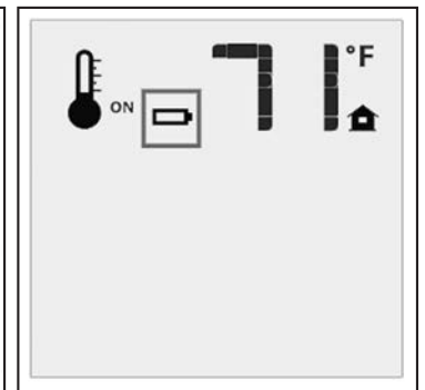
Figure 16: Low Battery Indicator.
