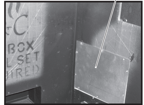
Figure 22: Access to firebox.
