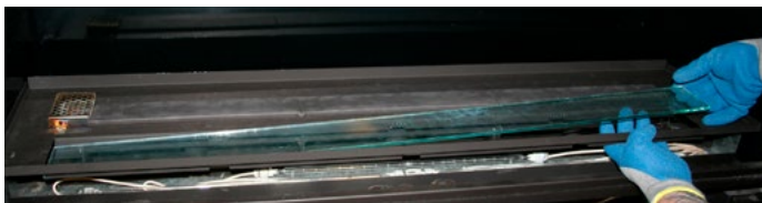
Figure 29. Remove the up-lighting glass from the burner tray.
