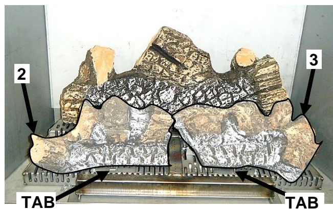
Step 3: Place LOG 2 and LOG 3 in between Rear and Front Burner Tube. Pull Logs up to the Tabs behind the Front Burner Tube.
