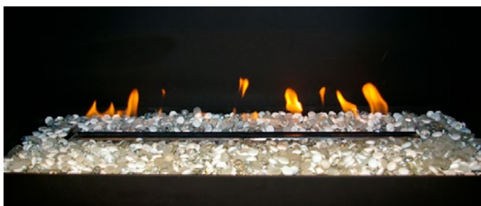
Figure 11a. Operating gas fireplace with firestones surrounding burner tray.
