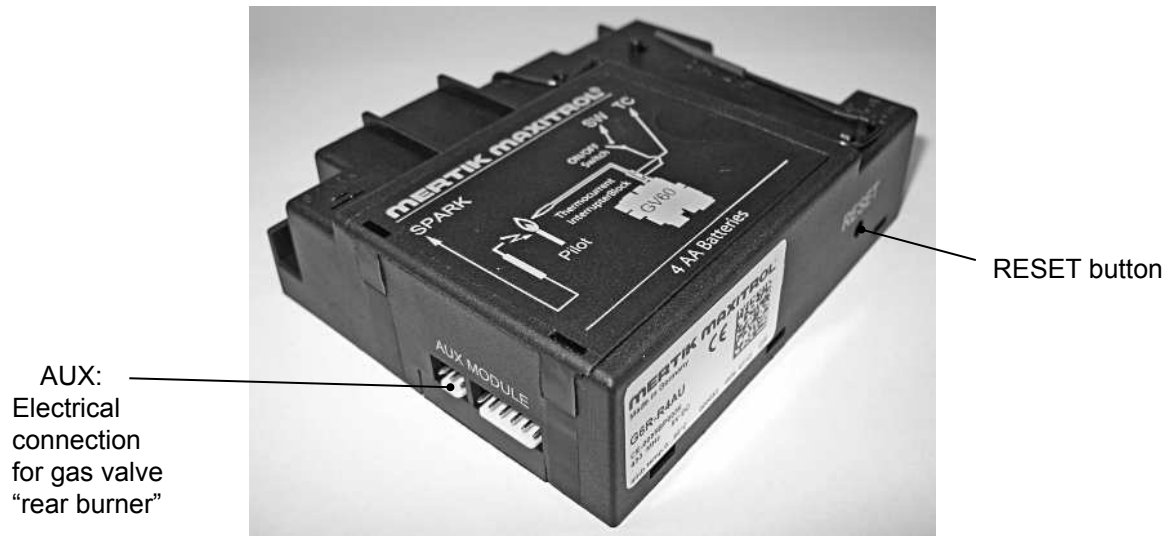
Figure 25: Receiver - AUX connection - RESET button
