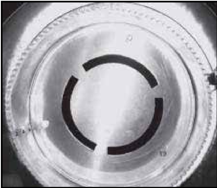
Figure 10: Restrictor for the TC30.
