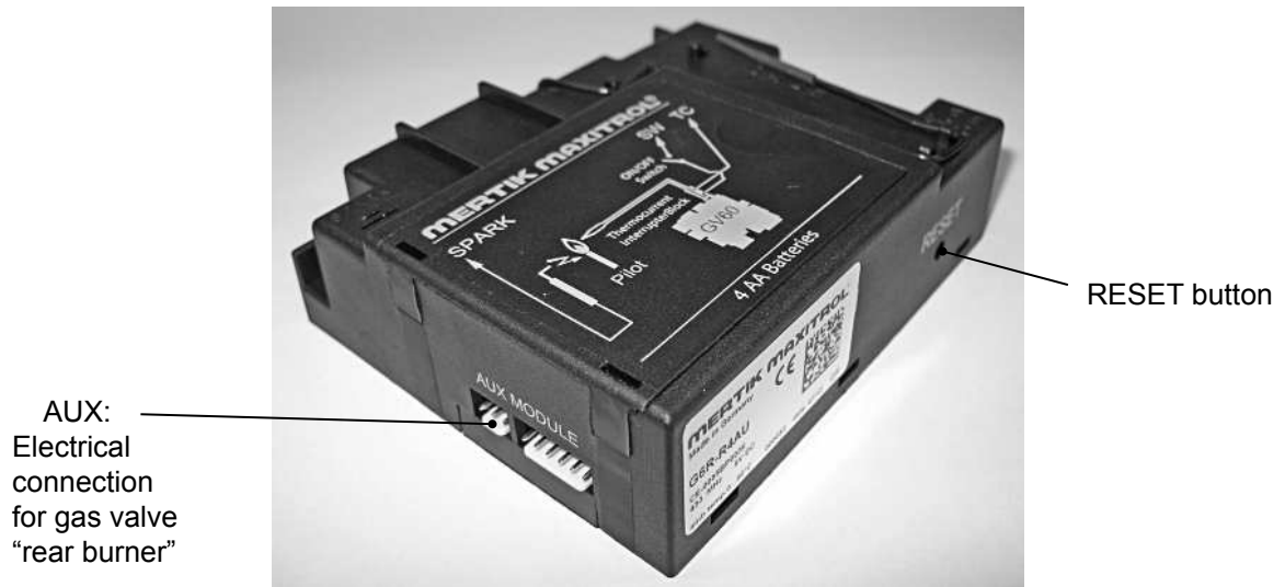
Figure 20: Receiver - AUX connection - RESET button
