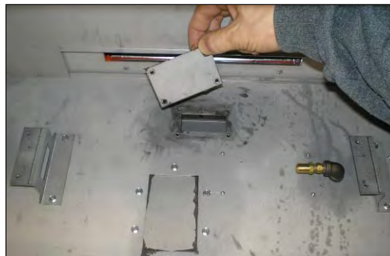
STEP 1: Remove false bottom to expose burner tube. Remove burner tube and cover plate as above. Remove old sealant from opening.
