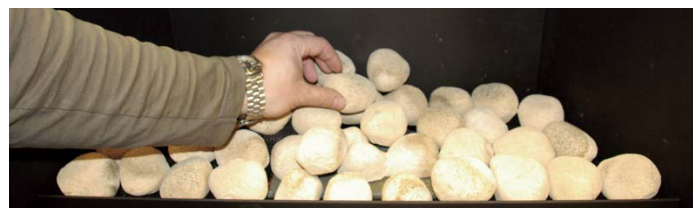
Figure 23.q Place the fourth Top faux Rock on top of the previous (2) two Rocks.
