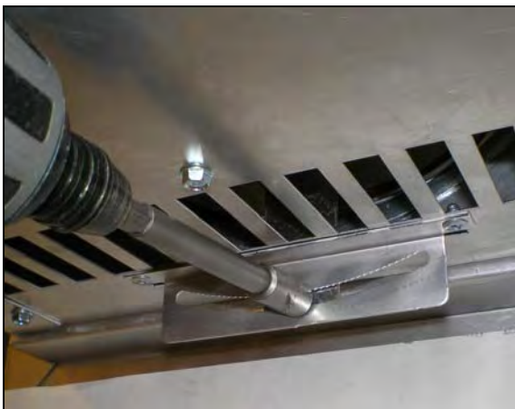
Once the desired draw has been set, re-tighten adjuster screw.
