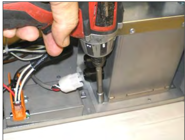
Reposition Lamp Transformer housing. Install Power Vent Control Module as shown.
