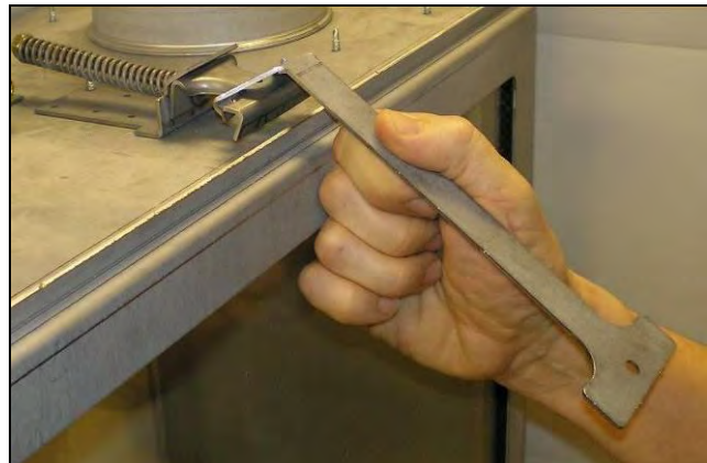
Step 6: Release Tool from Latch.
