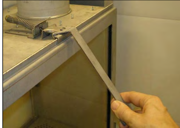
Step 2: Grasp Latch with Tool.
