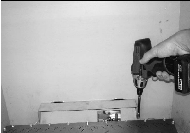
Step One: Remove Log Holder.
