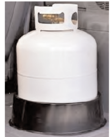
The above photo shows an example of an approved LP cylinder retention device.
