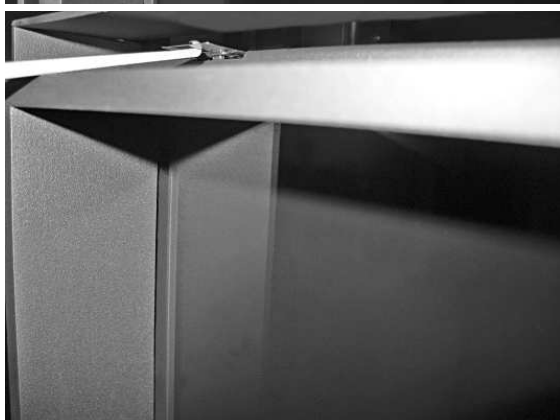
- With the hook, pull the thin, metal spring strips on the top left and right from the studs on the frame.
