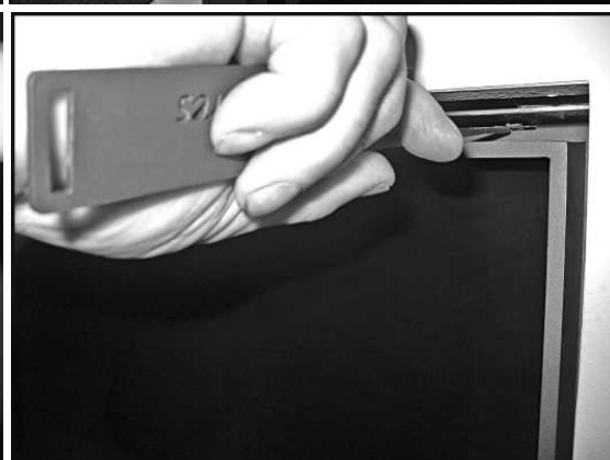
- With the hook, pull the thin, metal spring strips on the top left and right from the studs on the frame.
