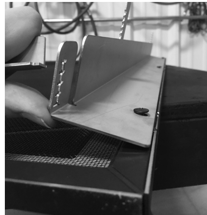
Figure 4.11, Screw Location on Hanging Bracket
