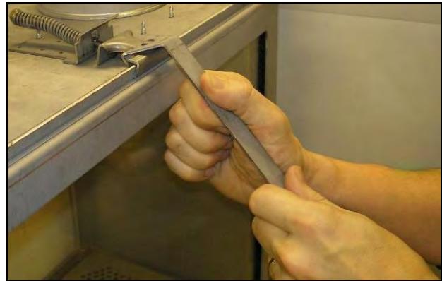
Step 4: Draw Latch forward with other hand.
