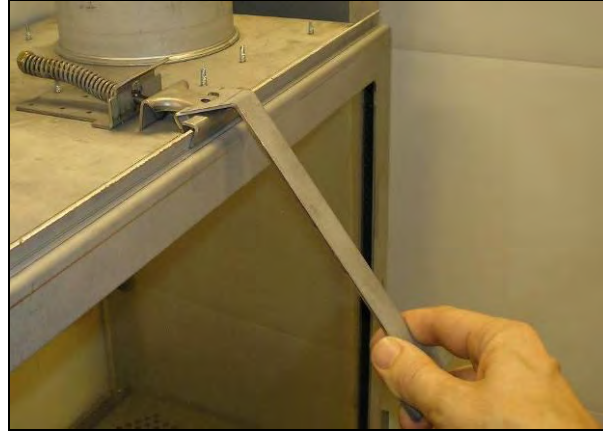
Step 2: Grasp Latch with Tool.
