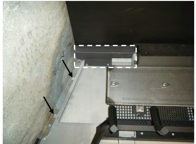
Step Five: Reinstall Liner Supports and Screws.
