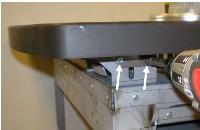
1. Remove the [2] screws from the top mount bracket on each side of the appliance.
