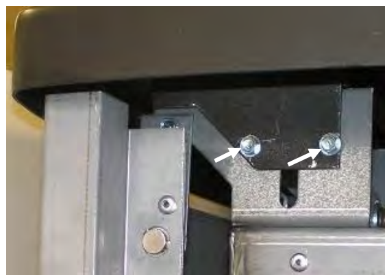
3. Once lower hooks are engaged, insert and tighten [1] DT Screw into mounts on upper sides of Door Face. Replace the [2] screws from the top mount bracket on each side of the appliance.
