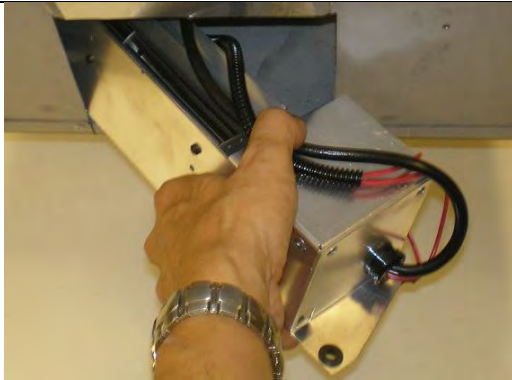
Slide Z46FK Fan Kit into opening.
