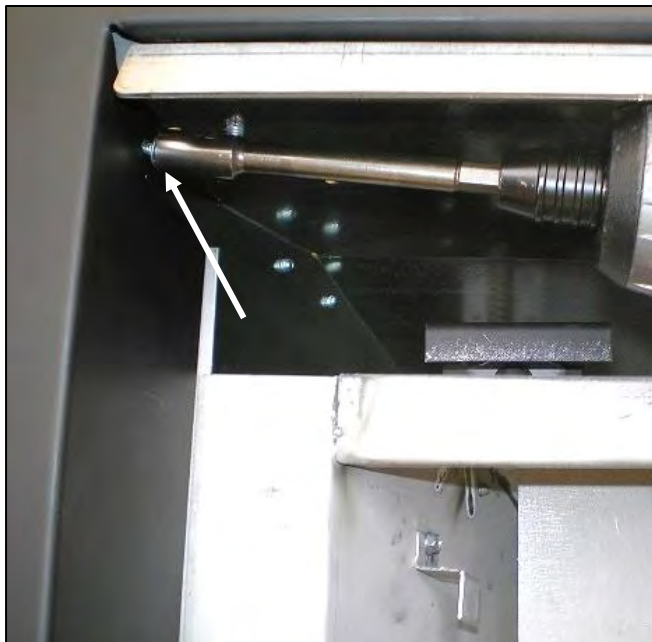
Step 3 (illustrated): Install screws in top corners.
