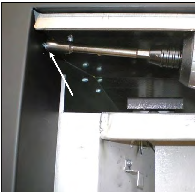
Step 3 (illustrated): Install screws in top corners.
