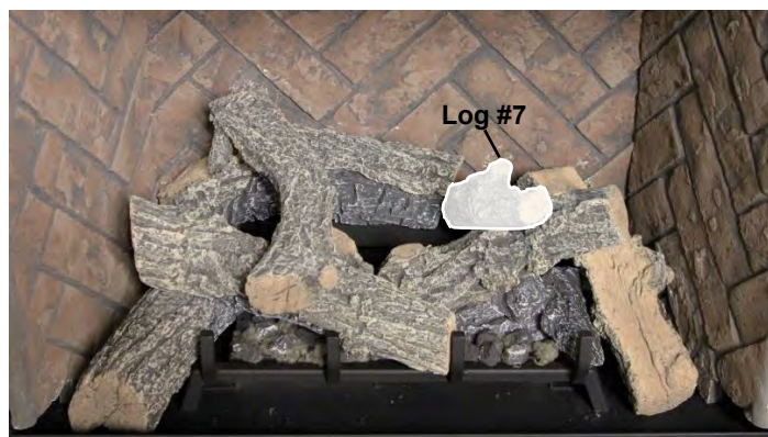
Step 8: Place Log #7 onto empty spot on Rear Log Holder and onto Log #4 making sure to position between the end flame and center flame evenly. There should be no impingement of flames or sooting may occur.
