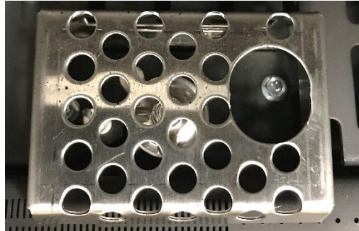
*Pilot Shield should be visually inspected monthly for signs of deterioration due to flame exposure. Replace if necessary.
