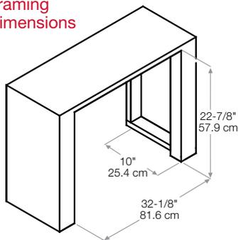
**Note:** The fireplace needs to be installed to ensure 35 in<sup>2</sup> (226 cm<sup>2</sup>) of intake air, into the back of the unit, on a continuous basis.
