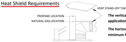
The vertical vent heat shield must be installed for EVERY type of venting application.
