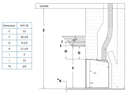
\*Required when installing on combustible flooring using floor protector (#RT29-FLP)
