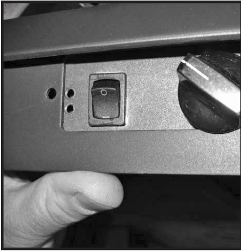
Figure 18: Reinstalling the Speed control assy.
