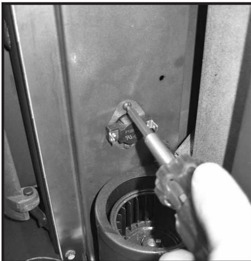
Figure 22: Removing thermal switch.
