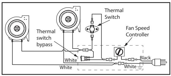
Figure 10: Wiring Diagram - Insert LE.
