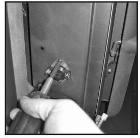
Figure 23: Relocating thermal switch to left side.
