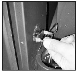
Figure 16: Disconnecting thermal switch.
