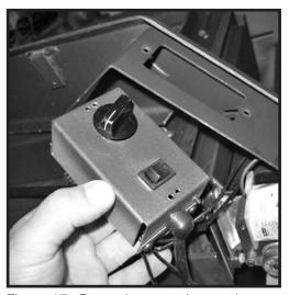
Figure 17: Removing speed control assy.
