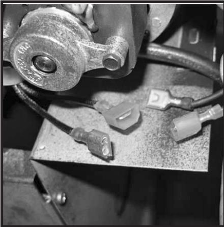
Figure 15: Disconnecting fan wires.
