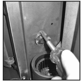
Figure 22: Removing thermal switch.
