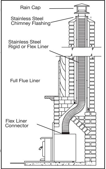
Figure 7: Full flue liner.
