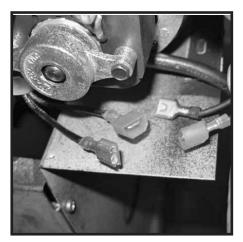
Figure 15: Disconnecting fan wires.
