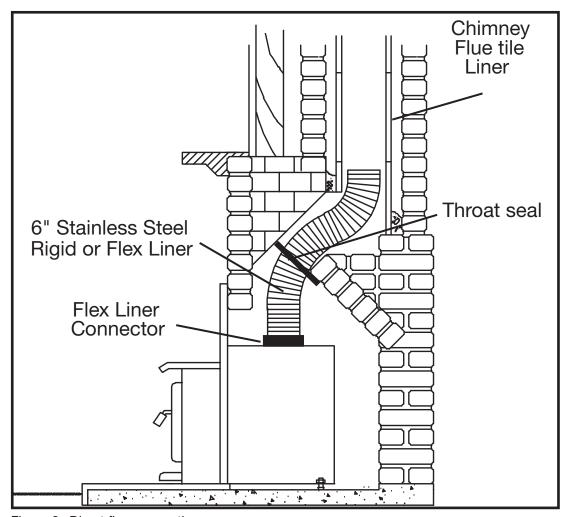
Figure 8: Direct flue connection.
