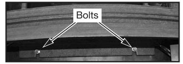
Figure 18: Bolts securing ash lip to firebox.
