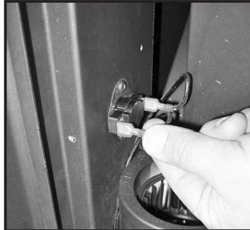
Figure 16: Disconnecting thermal switch.
