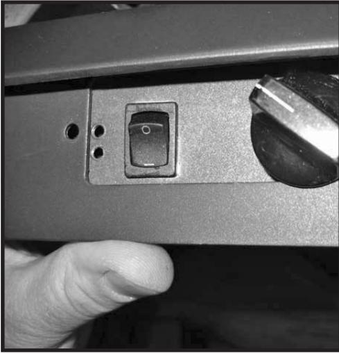
Figure 20: Reinstalling the Speed control assy.
