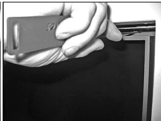
- With the hook, pull the thin, metal spring strip on the top middle from the stud on the frame.
