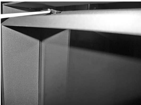
- With the hook, pull the thin, metal spring strip on the top middle from the stud on the frame.
