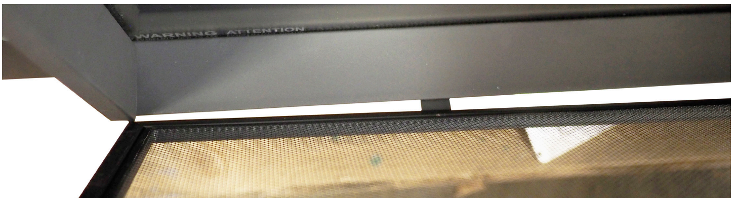
Figure 51 Rest the bottom of the screen on the 3 tabs that are under the trim. Push the screen into position so that the exposed magnets come in contact with the screen frame.
