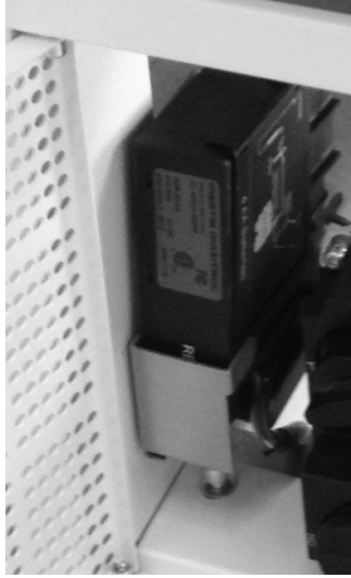
Figure 27 Receiver in Wall Access Door
